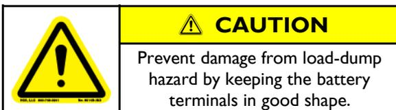
Load dump occurs when the car battery is disconnected while the engine of the car is still running. This can lead to voltage pulses as high as 70 volts, about six times the nominal battery voltage. This can be prevented by keeping your car in good condition. Especially the battery terminals need annual inspection and maintenance against corrosion.
