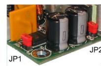
Jumper 2 [JP2] is hidden at the corner of the heatsink. This jumper selects the default shutdown delay. When placed, the shutdown signal will be issued about 15 seconds after the switch line is deactivated. When removed, this shutdown signal is delayed by approximately 15 minutes.
